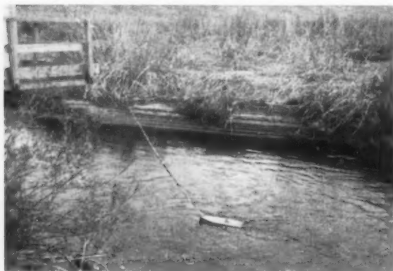
WATER is continually tested for pH at station house. pH electrodes are on small boat connected to chart meter above.
